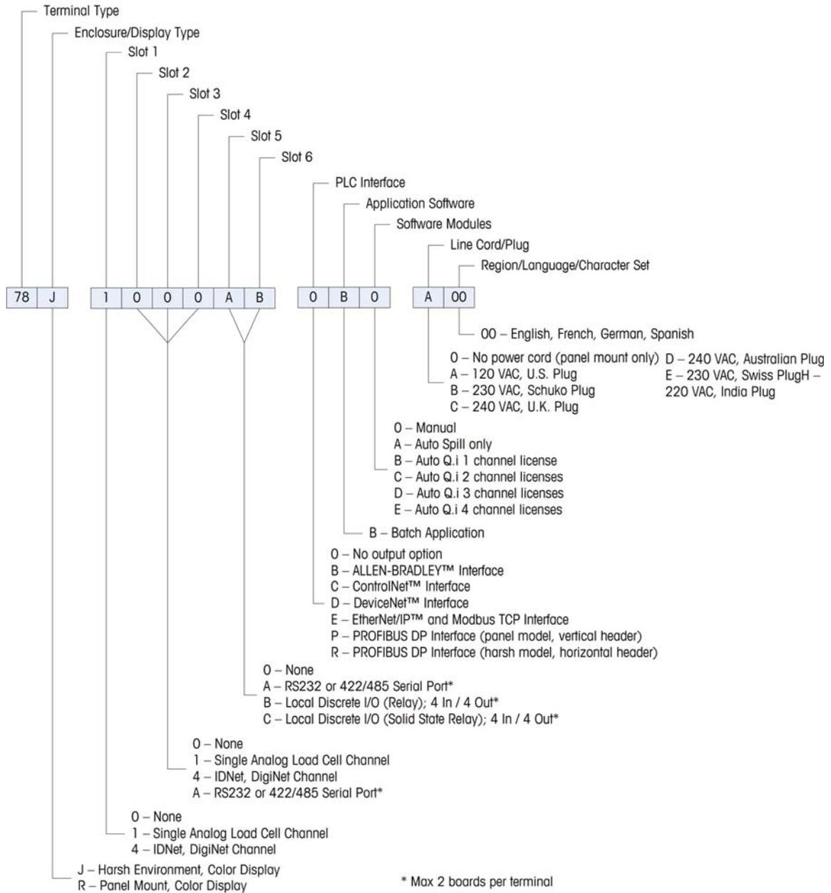
Figure 1-5: IND780batch Model Identification Numbers
